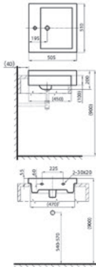
51cm Semi-Recessed Basin (1-Hole) Size: 510x505x200mm Material: Vitreous china 51公分半嵌盆(单孔) 尺寸: 510x505x200mm 材质: 陶瓷
