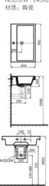
70cm Basin(1-Hole) + Semi Pedestal Size: NC2214W-1: 700x450x190mm NCE02W: 245X280X250mm Material: Vitreous china 70公分盆(单孔)+半底座 尺寸: NC2214W-1: 700x450x190mm NCE02W: 245X280X250mm 材质: 陶瓷
