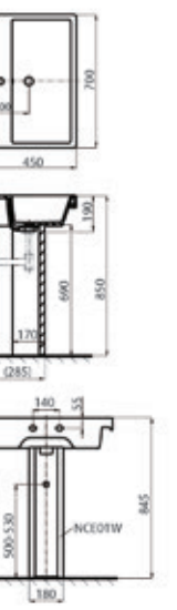
70cm Basin(1-Hole) + Pedestal Size: NC2214W-1: 700x450x190mm NCE01W: 180X170X690mm Material: Vitreous china 70公分盆(单孔)+底座 尺寸: NC2214W-1: 700x450x190mm NCE01W: 180X170X690mm 材质: 陶瓷
